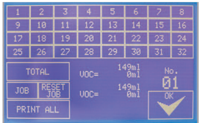
Consumption of up to 32 colours/materials (resin, catalyst and solvent) can be independently monitored for VOC content and material usage.
